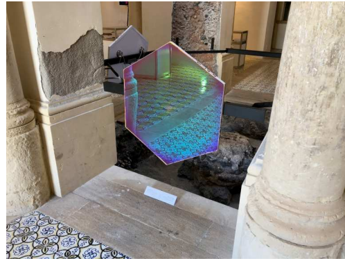
Fig. 4. The 85 cm hexagonal mirror of the Astri-Horn d’Arturo telescope at Serra La Nave
