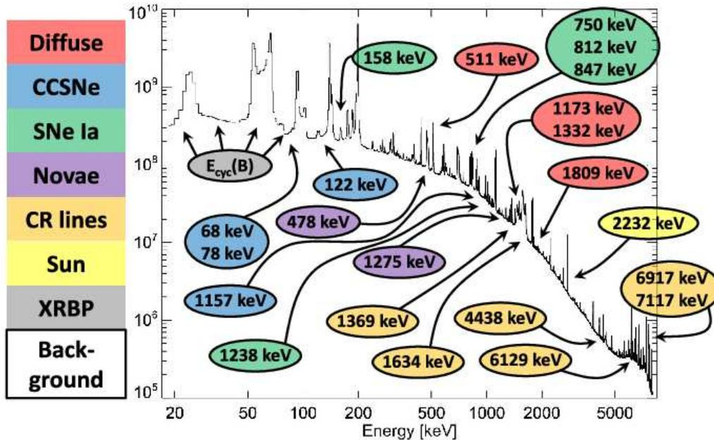
**Fig. 1.** SPI single event background spectrum (black histogram) from 16 mission years. In colours, prominent  $\gamma$ -ray lines from a variety of astrophysical sites are indicated. Note that there is substantial overlap between  $\gamma$ -ray lines from different source types. The indicated lines are either expected to be measurable or have already been detected and studied with INTEGRAL. See text for details.
