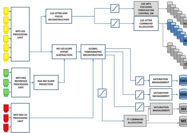
**Fig. 1.** Conceptual overall control loop diagram for MCAO mode configuration. The actuators depicted in grey belongs to the Telescope Control System. Functional blocks depicted in grey may not be commanded directly by the RTC.
