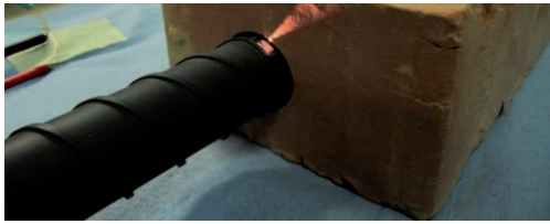
Fig. 3. Ma-MISS OH in the Drill tip
