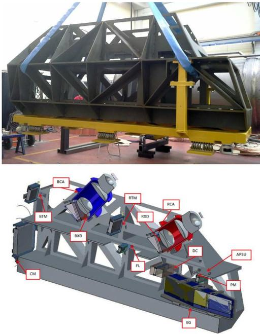
**Fig. 1.** Opto-mechanics of the ESPRESSO spectrograph. Top: optical bench as of July 2015. Bottom: scheme (APSU: Anamorphic Pupil-Slicer Unit, BCA: Blue Camera, BTM: Blue Transfer Mirror, BXD: Blue Cross-Dispenser, CM: Main Collimator, DC: Dichroic, EG: Echelle Grating, FL: Field Lens, PM: Field Mirror, RCA: Red Camera, RTM: Red Transfer Mirror, RXD: Red Cross-Dispenser.
