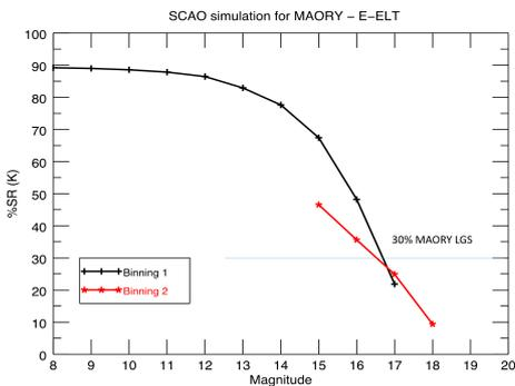
**Fig. 3.** SCAO Strehl ratio vs. R magnitude.
