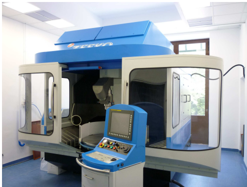
Fig. 1. The IRP1200 series machine in the clean room. The SMU is on the side of the machine, on the left. The SMU feeds the polishing process with recirculating pumped slurry maintained at constant temperature. An integrated density sensor monitors the specific gravity of the slurry.
