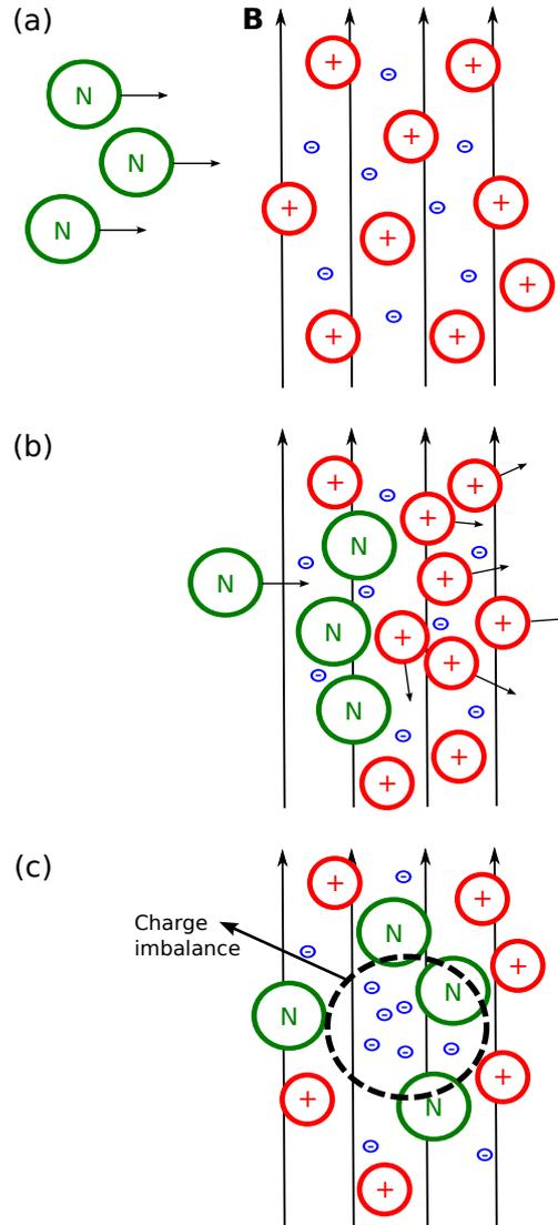
**Fig. 1.** The Alfvén ionization process: (a) A constant stream of neutral gas impinges on a low-density localized, magnetized plasma; (b) The inflowing neutral atoms collide with and displace the plasma ions; (c) the displaced ions leave behind a significant charge imbalance that accelerates electrons to energies sufficient to ionize the local gas via electron-neutral impact ionization.
