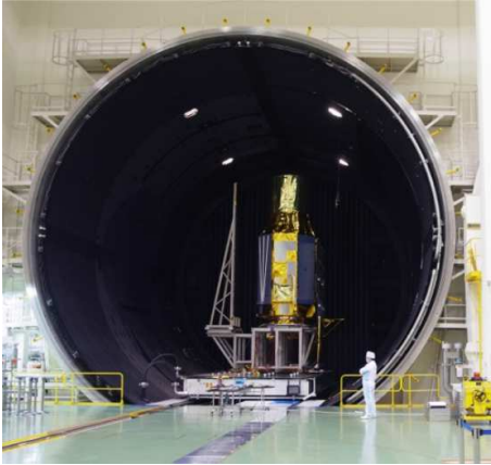
Fig. 3. The TTM model of the ASTRO-H satellite. Structures such as FOB, side panels and base plates are flight parts.
