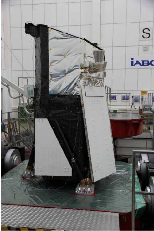
Fig. 6. The eROSITA qualification model on the shaker for vibration tests
