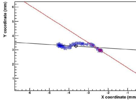
**Fig. 1.** Example of a photoelectron track imaged by the GPD filled with an Ar 70%–DME 30% gas mixture at the pressure of 2 bar. The black cross is the barycentre of the charge distribution, the black solid line is the main axis of the track, the red cross is the absorption point and the red solid line is the emission direction of the photoelectron.
