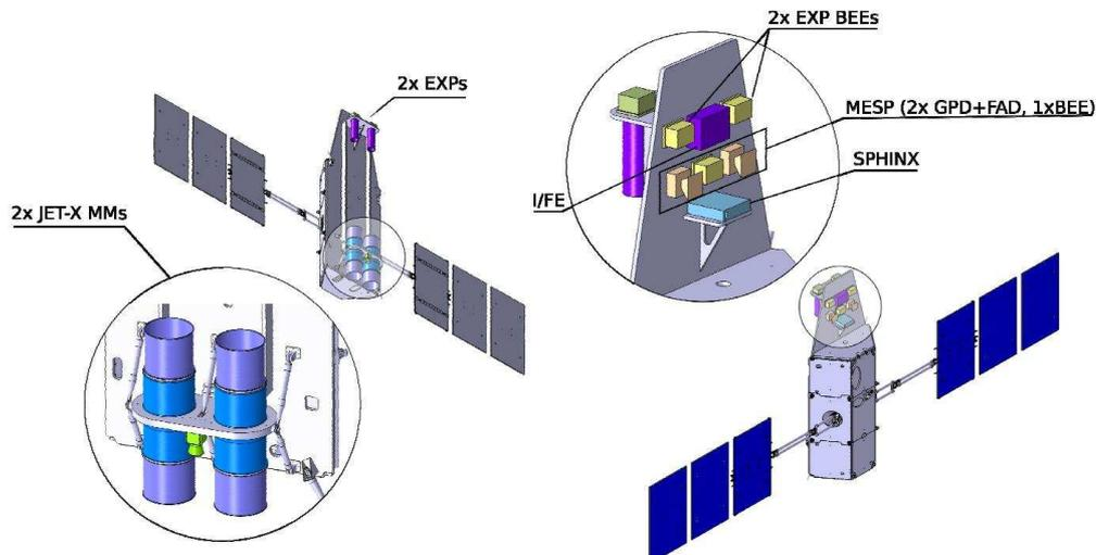
**Fig. 3.** XIPE spacecraft. The EXP (Efficient X-ray Photoelectric Polarimeters) units are the GPDs for polarimetry of non-solar sources, the MESP (Medium Energy Solar Polarimeter) units are the GPDs for solar flares observations.
