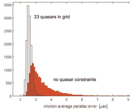
**Fig. 1.** Distributions of mission-average parallax error of the SIM interferometer project with and without 23 ICRF quasars used as hard constraints in the global solution, but with otherwise the same input parameters. The remarkable improvement in the expected parallax accuracy and the tightening of the uncertainty of the mission outcome arises from the reduced propagation of accidental zonal errors in low-order spherical harmonics.
