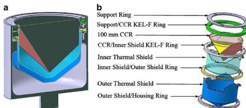
Fig. 5. Views of current design of the MoonLIGHT/LLRRA21 CCR: (a) fully assembled; (b) exploded view with its internal mounting elements and outer aluminum housing.
