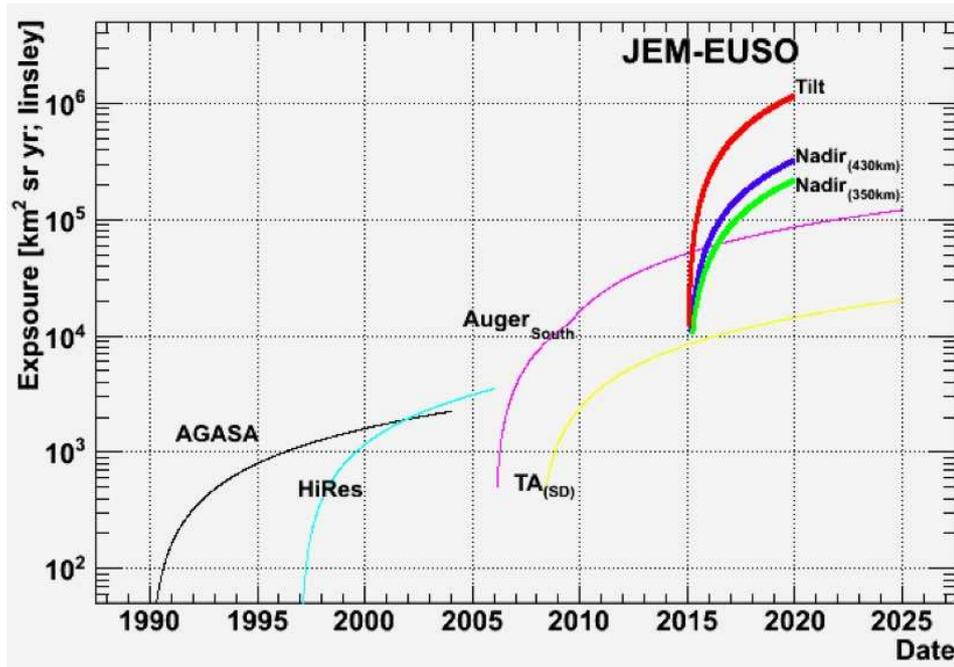
**Fig. 2.** Expected cumulative exposure of JEM-EUSO (Thick blue curve). For comparison, the evolution of exposure by other previous and presently running UHECR observatories is shown (JEM-EUSO Internal Report, Purple Book, 2010).
