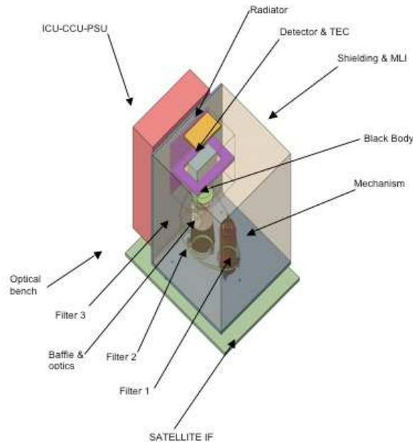
**Fig. 3.** Preliminar design of the JEM-EUSO Infrared Camera (JEM-EUSO Internal Report, Purple Book, 2010).
