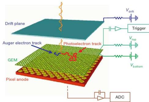
**Fig. 1.** Principle of operation of the Gas Pixel Detector (Costa *et al.* 2001).
