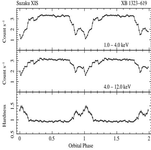
**Fig. 3.** Background-subtracted XIS lightcurve of XB 1323-619 folded on the best-fit orbital period of 2.928 hr obtained by dip analysis. Top panel: in the energy band 1.0- 4.0 keV; middle panel in the band 4.0 - 12.0 keV; the lower panel shows the hardening in dipping in the ratio of the two energy bands.
