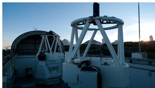
**Fig. 1.** The two STELLA telescopes on Tenerife: To the left the STELLA-I telescope, which feeds the spectrograph now, but will host an imaging instrument from 2010 on. To the right the STELLA-II telescope, which will feed the spectrograph from 2010 on.
