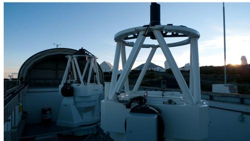
**Fig. 1.** The two STELLA telescopes on Tenerife: To the left the STELLA-I telescope, which feeds the spectrograph now, but will host an imaging instrument from 2010 on. To the right the STELLA-II telescope, which will feed the spectrograph from 2010 on.
