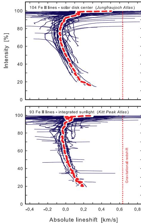
**Fig. 2.** Fe II bisectors in spectra of solar-disk center and of integrated sunlight. Each thin curve is the bisector of one spectral line; the thick dashed is their average. The vertical scale denotes the intensity in units of the spectral continuum, while the dotted line marks the wavelength expected in a classical 1-D model atmosphere, given by the laboratory wavelength, displaced by the solar gravitational redshift.
