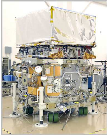
Fig. 2. The GLAST LAT and GBM during spacecraft integration at General Dynamics, in December 2006. (Credit: NASA/General Dynamics Advanced Information Systems).
