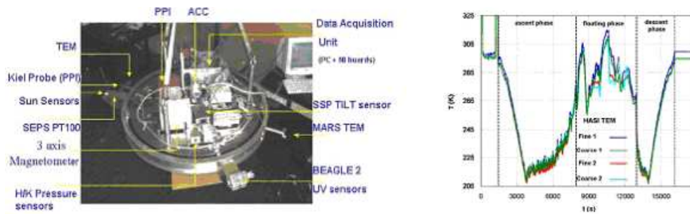
Fig. 4. Instruments of the HASI probe and results of the experimental campaign.
