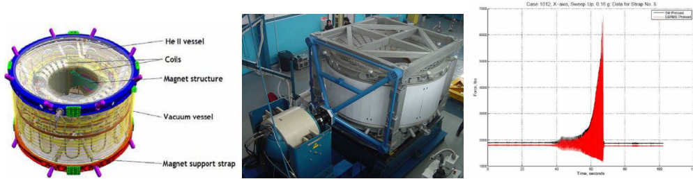
Fig. 4. Left: Schematic drawing of the AMS Magnet. Center: The Stress Test Article mounted on the SERMS slip table. Right: Registered force on one strap as a function of time during the x-axis vibration test.
