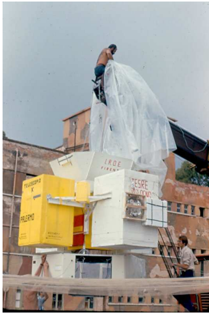
Fig. 6. The payload of the 1976 Italian transatlantic experiment. The total weight was about 1500kg plus flight service module and ballast. The main experiment were from LAS-CNR (Rome), ITESRE-CNR (Bologna), IROE-CNR (Florence), IFCAI-CNR (Palermo) plus a few small piggy-bag. The man on top the crane arm is Dr. Marco Malavasi, at that time the Director of the Trapani-Milo Facility. The pink net, visible in the bottom part of the payload, is the virtual-ground of about 8 m diameter necessary to operate the HF transmitter during the flight (Courtesy of F. Giovannelli).
