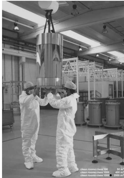
Fig. 1. Preparation of a gold-coated mandrel for Nickel electroforming at Media Lario Technologies .
