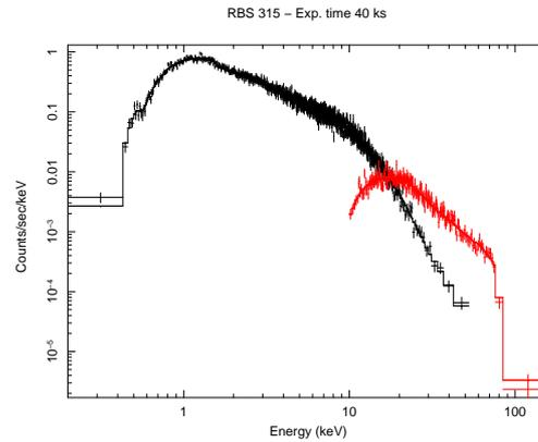
**Fig. 6.** Simulated *SIMBOL-X* spectrum (black: low energy instrument, MPD; red: high-energy instrument, CZT) of RBS 315 assuming the parameters of the best fit model reproducing the *Suzaku* observation reported in Fig.5 and with an exposure time of 40 ksec s. The source is clearly detected up to 100 keV and the spectral parameters can be derived with an uncertainty below 10%.
