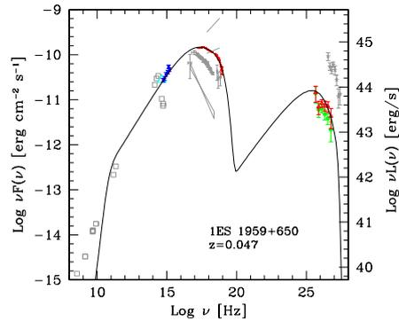
**Fig. 2.** SED of the BL Lac object 1ES1959+650 assembled with simultaneous optical-UV, X-rays (*Suzaku*) and TeV (green: observed, red: corrected for the intergalactic absorption) data taken in May 2006 (*MAGIC*). Grey points show historical data. The solid line shows the one-zone synchrotron-inverse Compton model reproducing the data (Hayashida et al. 2007).
