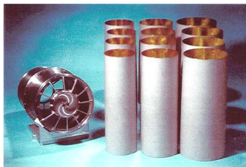
Fig. 1. Mirror shells and mandrels developed for making the X-ray optics module aboard Swift.
