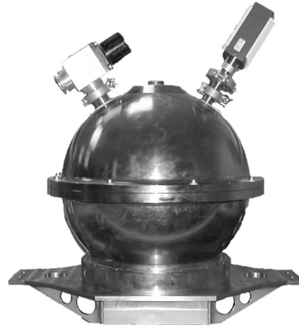
Fig. 2. LBC Red cryostat with vacuum sensor valve
