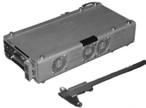
Fig. 3. LBC CCD controller electronics box
