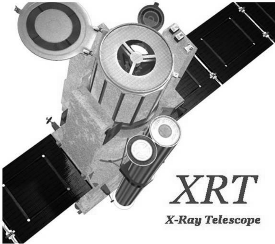
Fig. 1. The X-Ray Telescope (XRT) is one of the main instruments on board the Hinode satellite.
