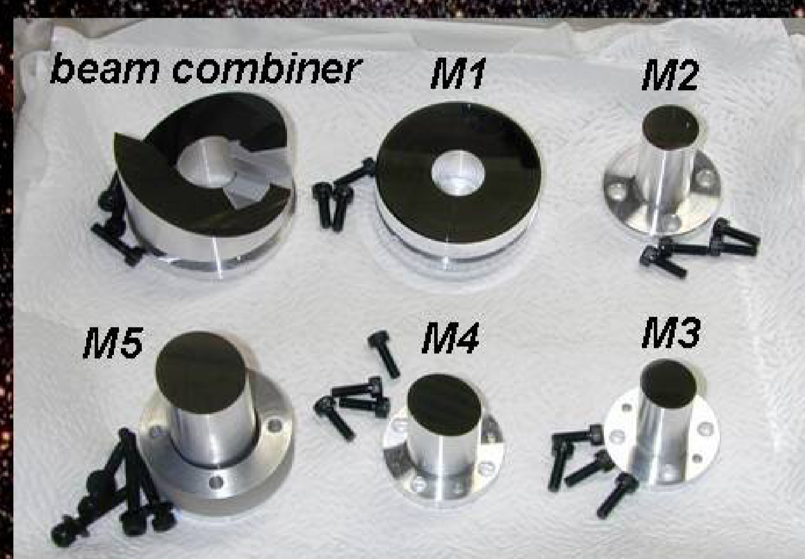
Mirrors for Nano-JASMINE telescope. Their reflecting surfaces are shaped directly with diamond turning machine.
