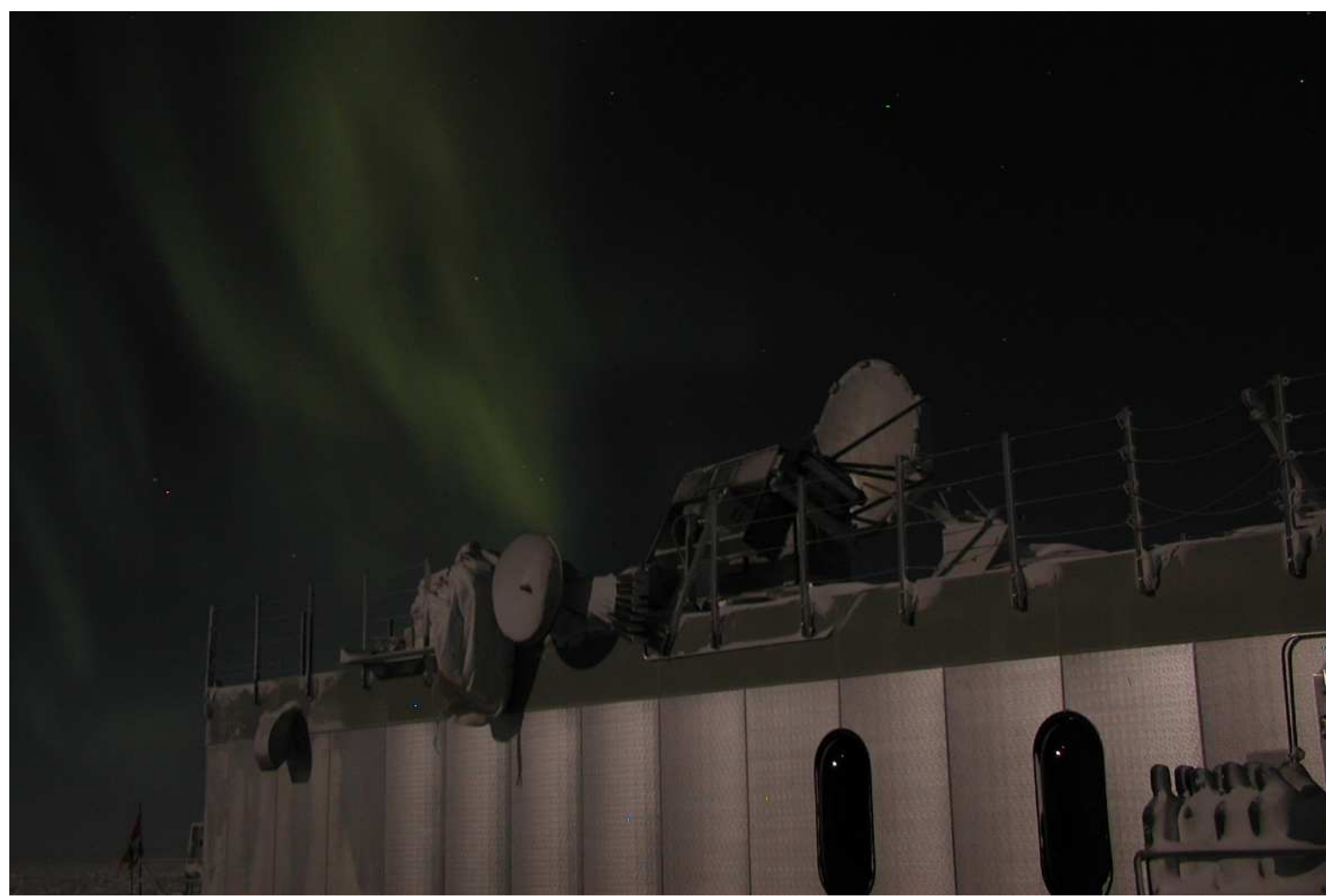
Figure 1: Above is a picture of AST/RO in August 2001 with the aurora overhead. AST/RO [Stark et al. 2001] is a 1.7 m diameter, offset Gregorian telescope capable of observing at wavelengths between 200 \mu m and 1.3 mm. Located only 1 km from the geophysical South Pole, and the NSF's Amundsen-Scott South Pole Station, the author (CLM) spent two full years in 2001 & 2003 collecting data for this and other projects.
