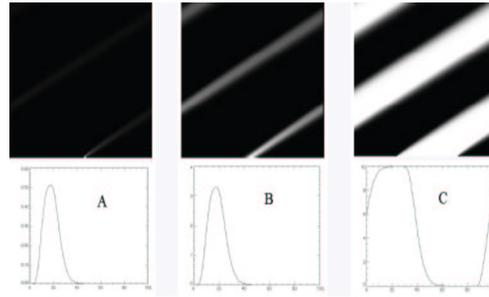
**Fig. 3.** Ray intensity on the domain (upper panels) and intensity profiles at the top of the grid (lower panels) for three different boundary conditions at the bottom: A) delta function; B) Gaussian function; C) step function.
