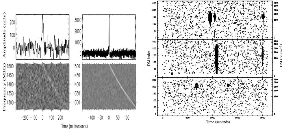
**Fig. 2.** The left panel shows two examples of a RRAT pulse, a strong single pulse (top) and the dedispersed time series across all frequency channels (bottom). The signal is clearly broadband and the dispersion sweep is as expected for a signal of astrophysical origin. The right panel shows DM index (left y-axis) and DM value (right y-axis) vs. time for three different RRAT detections. The size of the circle is proportional to the signal-to-noise ratio of the pulse. McLaughlin et al. (2005)
