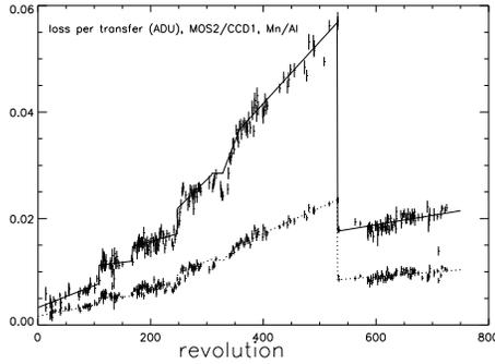
**Fig. 1.** Evolution of the CTI for the MOS2 central CCD, expressed as ADU signal losses per transfer, at the two energies of the calibration source,  $AlK_{\alpha}$  (1487 eV) and  $MnK_{\alpha}$  (5896 eV)
