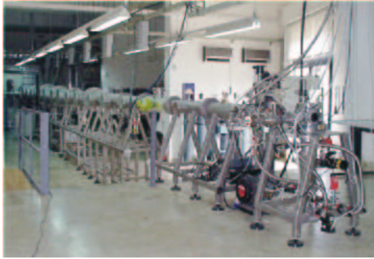
Fig. 1. The X-ray beam line of XACT. The X-ray source is in the forefront, on the right, the conical pipe is at the center of the image running, roughly, from right to left, with its supports, ports and all the technical equipments attaches. The test chamber with the clean room is in background, on the left.
