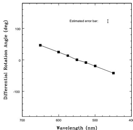
**Fig. 1.** Differential rotation angle as a function the input radiation wavelength, from a LCVR rotator.
