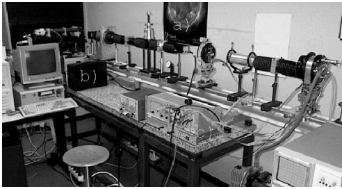
Fig. 1. The development system at the solar station. a) the APS detector, the acquisition PCI card is inside the PC; b) CCD-PI camera, similar to the present THEMIS-IPM cameras, and control electronic; c) CCD camera, former THEMIS-IPM camera, and control electronic.
