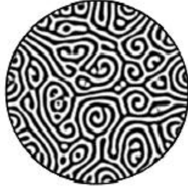
Fig. 2. Convective pattern, illustrated by contours of the thermal perturbation, arranged from Paul (2002). Dark features represent cool descending fluid and white features warm ascending fluid.
