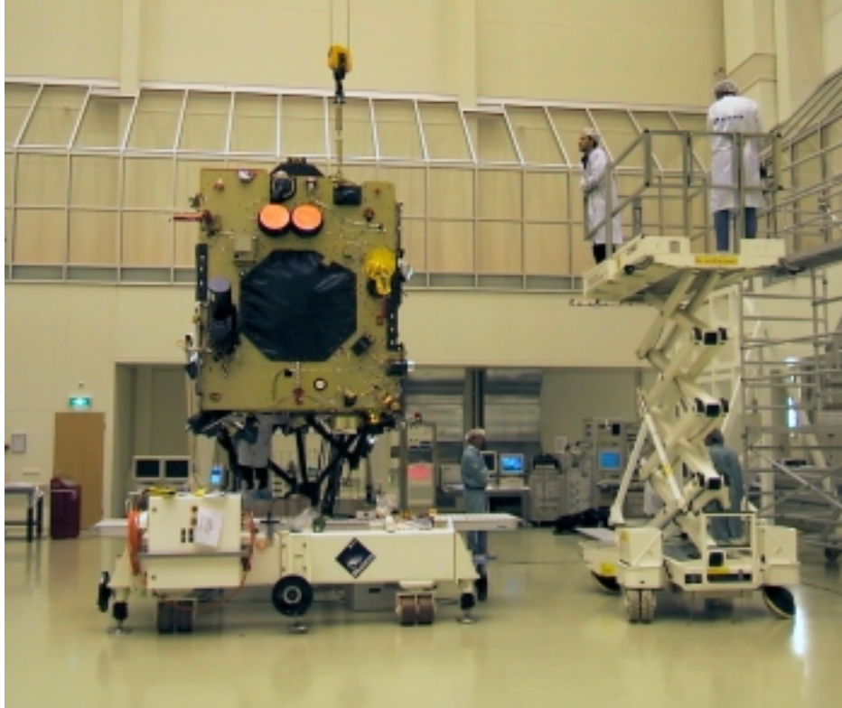
Fig. 2 – OSIRIS mounted on ROSETTA (upper edge) , the WAC on the left, the NAC on the right, the lander that is just visible (ESTEC, Dec. 2001).
