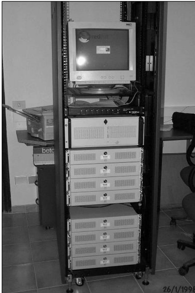
Fig. 2. The 8 nodes BEOWULF test cluster developed at Capodimonte Astronomical Observatory and available for the phase I of the project.
