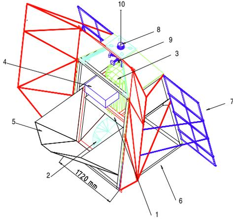
**Fig. 1.** The BOOMERanG payload. On the inner frame (1) are mounted the off axis primary mirror (2), the cryostat with the detection system (3), the analog electronics (4), the ground shield (5). On the outer frame (6) are mounted the sun shields, the solar panels (7), the azimuth pivot (8) with the flywheel (9). The pivot decouples the payload from the flight chain (10).
