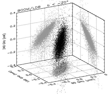
**Fig. 3.** 3D scatter plot of temperature fluctuations detected by BOOMERanG at 90, 150, 240 GHz. The measurements units are  $\mu K$  for thermodynamic temperature fluctuations of a 2.73K blackbody. The correlation shows that the bulk of the detected fluctuations has the spectrum of the CMB.
