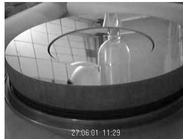
Fig. 2. The 30 cm primary of the TRT telescope realized by LIOPTICS.
