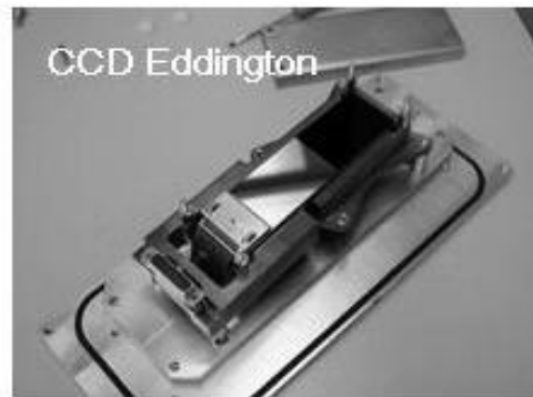
Fig. 2. One of the forecast CCDs for ESA space planetary transit search mission EDDINGTON
