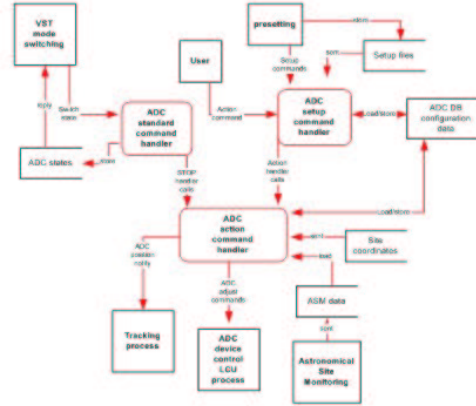
Fig. 1. The VST ADC control software data/commands flow diagram.
