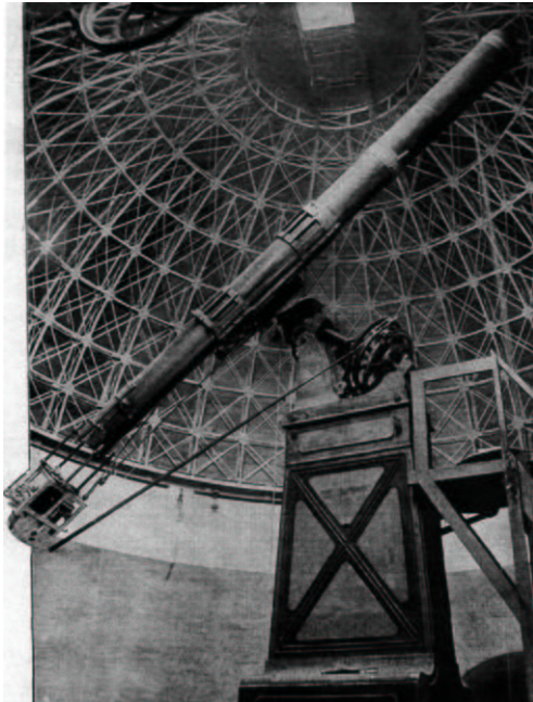
Fig. 6. Catania Observatory telescope, equipped with the same objective and same mounting of the Etnean Observatory, but with a wood pipe.
