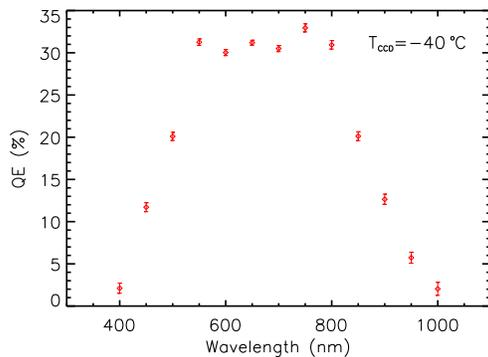
**Fig. 1.** Quantum efficiency of Kodak KAF-4202 CCD.
