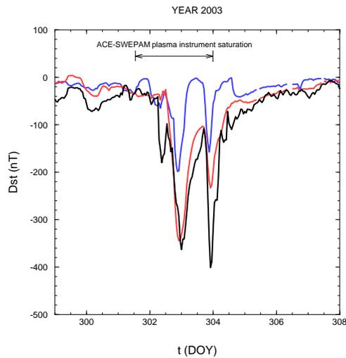
**Fig. 3.** Comparison between the Kyoto provisional Dst (black line), the IFSI ANN Dst (blue line) and the IFSI IMF ANN Dst (red line) between day 299 and day 308, 2003.
