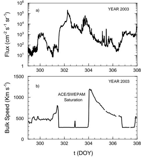
**Fig. 2.** Top panel: flux of protons of energy greater than  $1MeV$  observed by the geostationary GOES 11 satellite between day 299 and day 308, 2003. Bottom panel: Real time speed transmitted to the ground by the ACE SWEPAM solar wind plasma instrument for the same time period.
