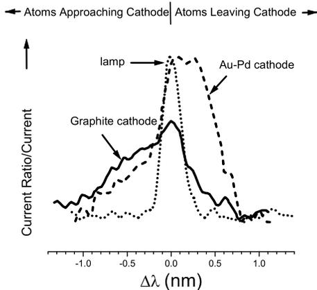
**Fig. 5.** Line profiles of  $H\alpha$  emission at 10 kTd from a discharge in hydrogen with AuPd and graphite cathodes (Petrović & Phelps 1991a; Petrović et al. 1992).
