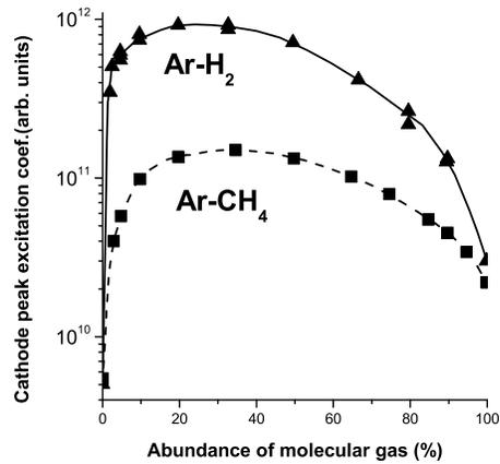
**Fig. 6.** Excitation coefficients at the cathode as a function of the abundance of molecular gas in argon (for hydrogen and methane mixtures with argon) (Jelenković et al. 1990; Petrović & Phelps 1991b). Measurements were made at 1 kTd at 150 mTorr and  $V=190$  V for hydrogen and 2 kTd, 100 mTorr and 260 V for methane mixtures.
