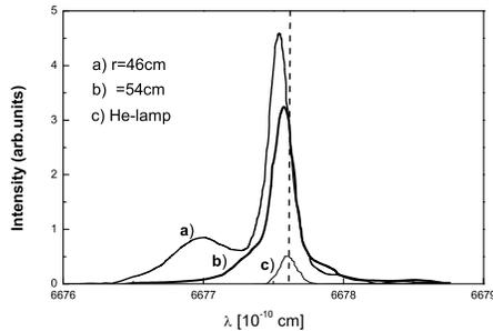
**Fig. 10.** He singlet line (667.8 nm) profiles from a fusion reactor discharge in helium (Bogen et al. 1989) at two positions (a-b) of the limiter and also including a spectral He lamp (c).
