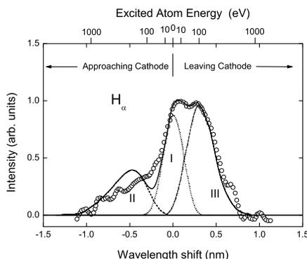
**Fig. 3.** Doppler broadened  $H\alpha$  profile at 10 kTd from a discharge in hydrogen with AuPd cathode (Petrović et al. 1992).
