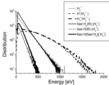
**Fig. 8.** Energy distribution of fast ions and fast neutrals in a hydrogen discharge at 10 kTd. The results are consistent with Doppler profiles and fast neutral excitation.
