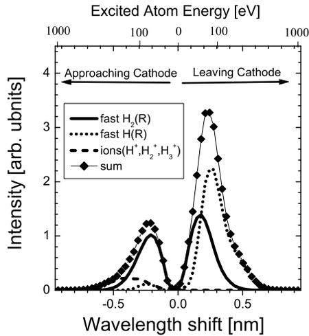
**Fig. 9.** Balmer  $H\alpha$  line profile obtained from the Monte Carlo simulation in a hydrogen discharge at 10 kTd (all conditions were the same as in the actual experiment).
