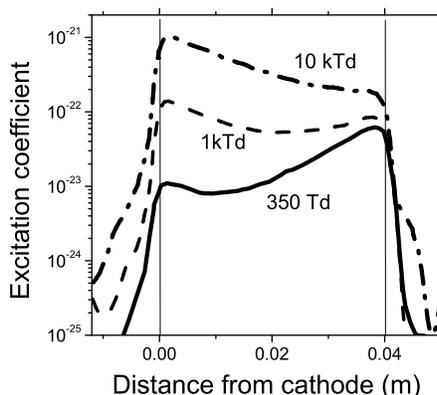
**Fig. 2.** Spatial emission profiles absolutely calibrated to the excitation coefficients for Townsend discharges in hydrogen (Petrović & Phelps 1991a).
