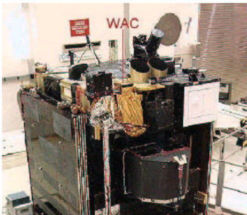
Fig. 1. OSIRIS mounted on ROSETTA (upper edge), the WAC on the left, the NAC on the center. Part of VIRTIS are seen on the right (photo taken in ALENIA, Dec. 2001).
