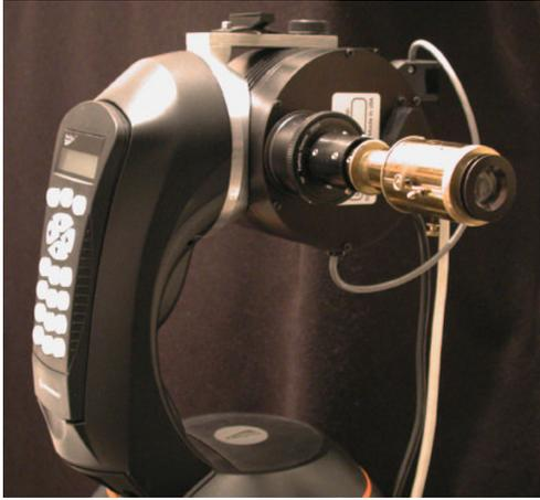
**Fig. 1.** The WASBAM-SSH spectrophotometer.
