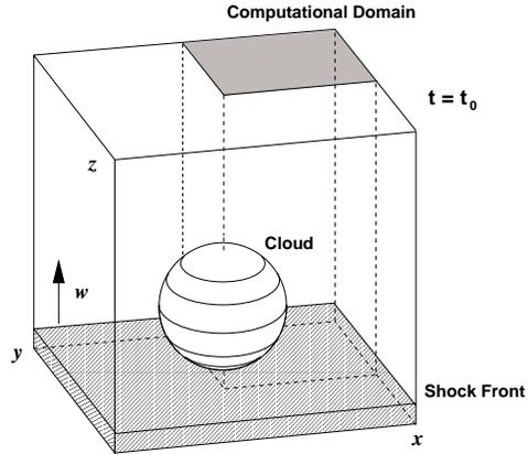
**Fig. 1.** Initial conditions for the shock-cloud interaction. The shock is moving upwards through the ISM with velocity  $w$ . The gray box marks our computational domain.
