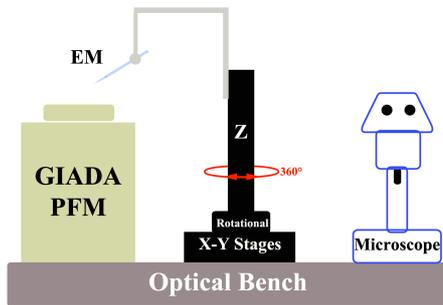
**Fig. 2.** Sketch of the setup used for the GIADA PFM calibration.
