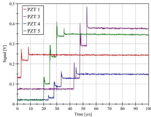
**Fig. 5.** Signals produced by IS sub-system as result of the impact of a forsterite grain particle (150-200  $\mu\text{m}$ ) shot by EM. The PZT2 signal is not acquired.
