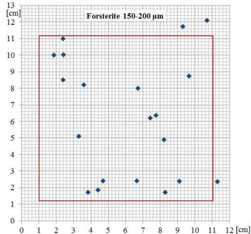
**Fig. 3.** Impact positions of twenty particles (blue points) of forsterite 150-200  $\mu\text{m}$  shot by the EM during a test on GIADA STM. The red square represents the sensitive surface of the Impact Sensor.
