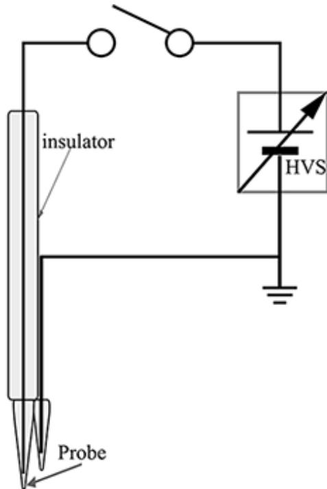
**Fig. 1.** Electric scheme of the Electrostatic Micromanipulator (EM) developed and realized in the “Laboratorio di Fisica Cosmica” – University Parthenope of Naples.
