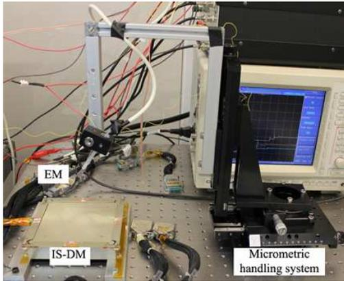
**Fig. 4.** Test using Electrostatic Manipulator on the IS-DM to verify that shot particles are detected by the sub-system.
